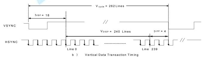
Figure 3 Data Transaction Timing in Serial RGB (8 bit) Interface (SYNC Mode)
