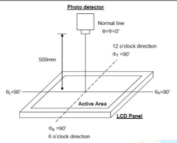
Fig. 8-2 Optical measurement system setup
