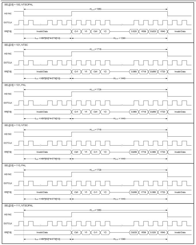
Figure 1 CCIR601 Horizontal Timing
