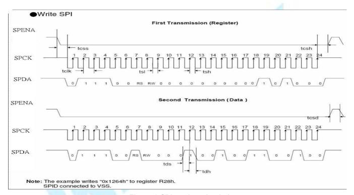
Figure 8 SPI read · write timing
