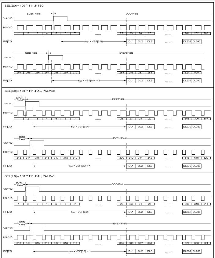
Figure 1 CCIR601 Vertical Timing
