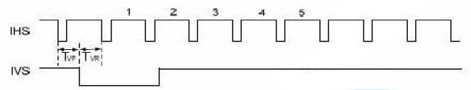
Figure 7 IHS and IVS timing waveforms
