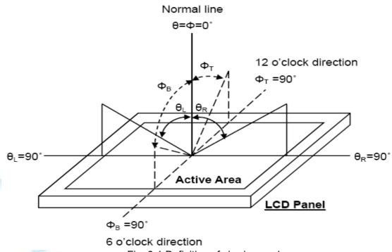
Fig. 8-1 Definition of viewing angle
