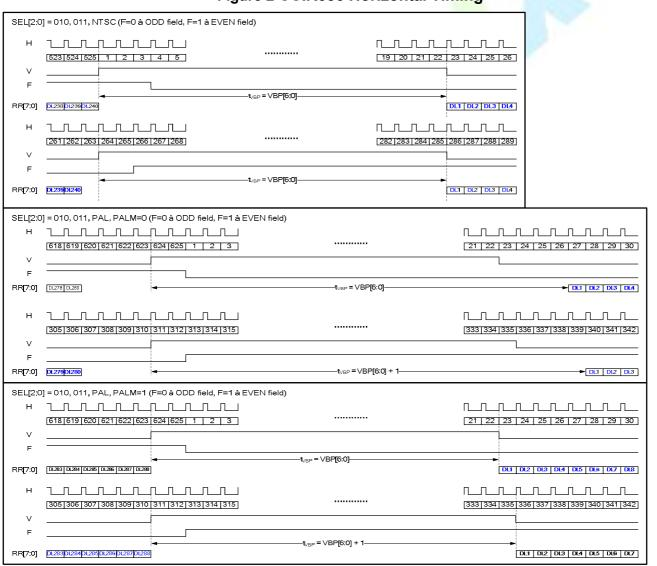
Figure 2 CCIR656 Vertical Timing
