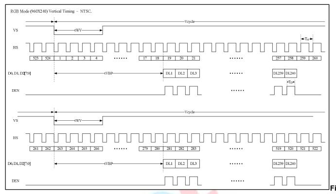
ure 3 Digital RGB NTSC mode Vertical Data Format for 262T<sub>H</sub>
