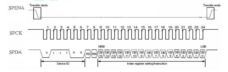
Figure 9 SPI timing
